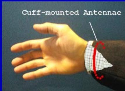
To achieve our goal of a "dynamically configurable wearable", we have developed a 1 foot range radio transceiver called "Foot-Bridge". Foot-Bridge allows us to connect companion devices to the wearable computer without wires. By mounting the antennae around the user's wrist or shirt cuff, we can detect devices being touched or held in preference to others in the vicinity. This allows automatic configuration of the wearable.
